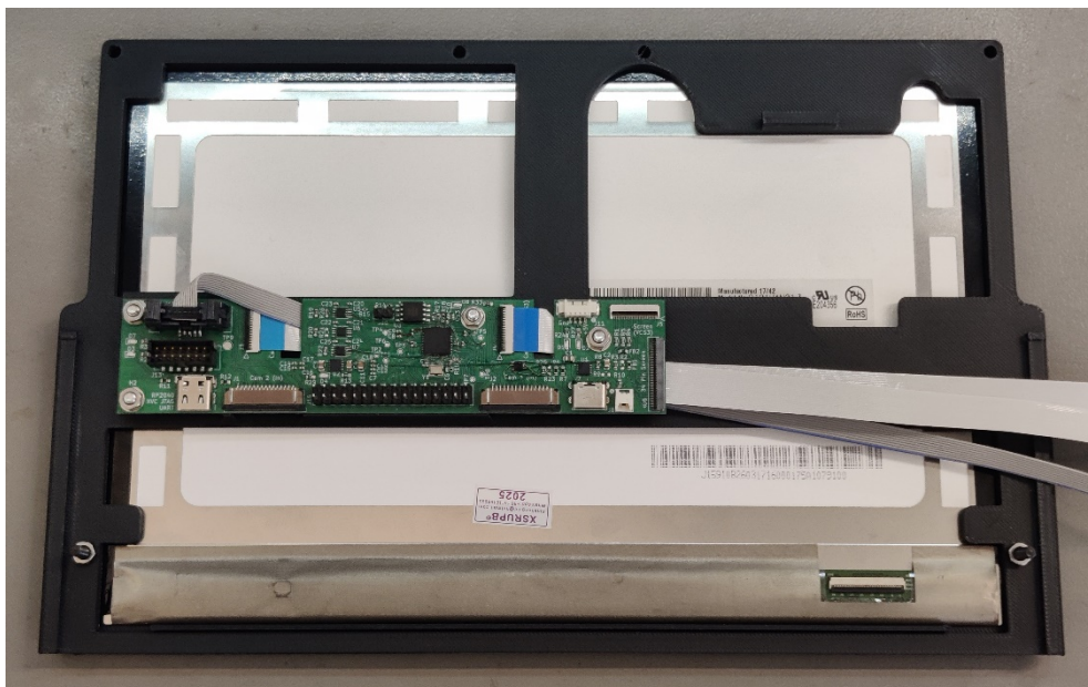
Figure 11: Rear view of Frame placed on Bezel, and attached using the bottom two holes
