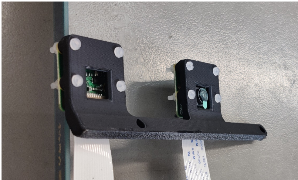
Figure 15: Front view of the Camera Mount with both cameras attached. Both cameras should be attached to the rear side of the Mount
