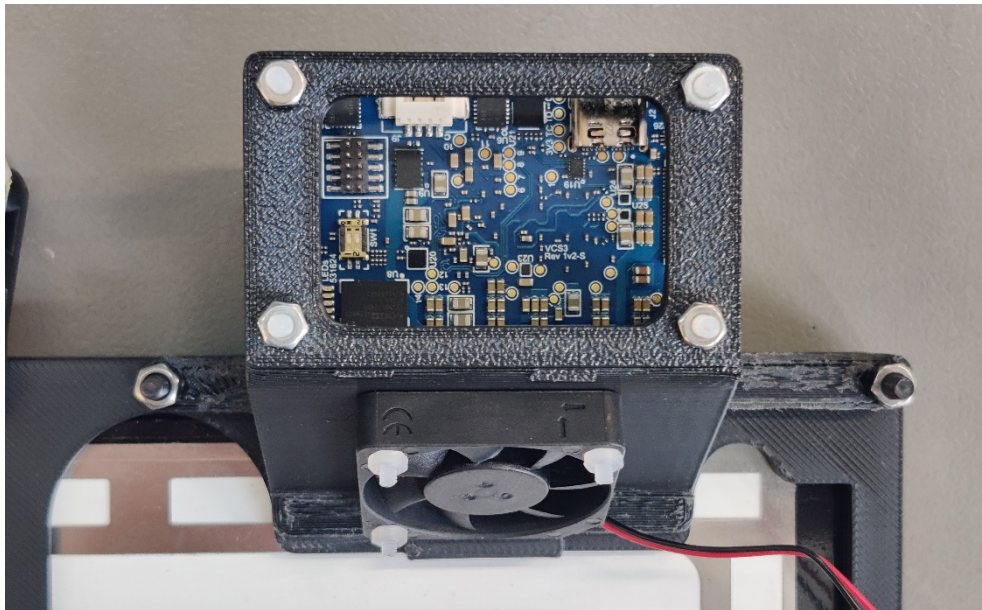
Figure 16: Rear view of VCS Holder attached to Frame
