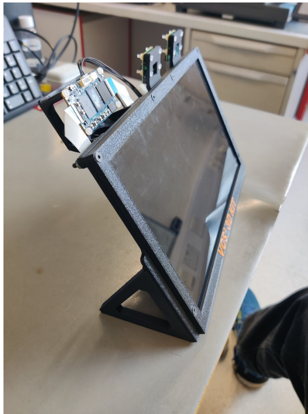
Figure 31: The 3D Kit sits at a 45 degree angle to the ground
