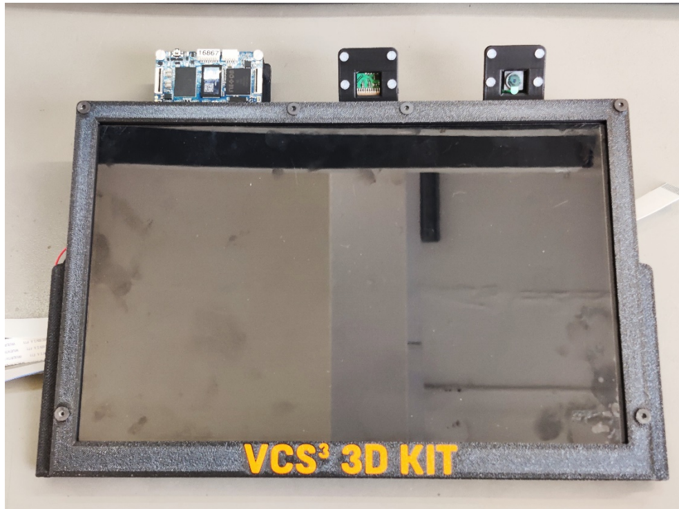
Figure 17: Front view of the 3D Kit with VCS³ Core and Camera Mount attached
