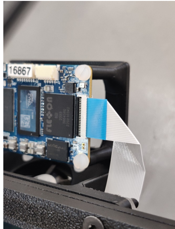
Figure 22: 22 pin FFC (7.97") connected to the front right connector on the VCS 3 Core. There is another 22 pin MIPI connector behind it, which is reserved for a camera connection
