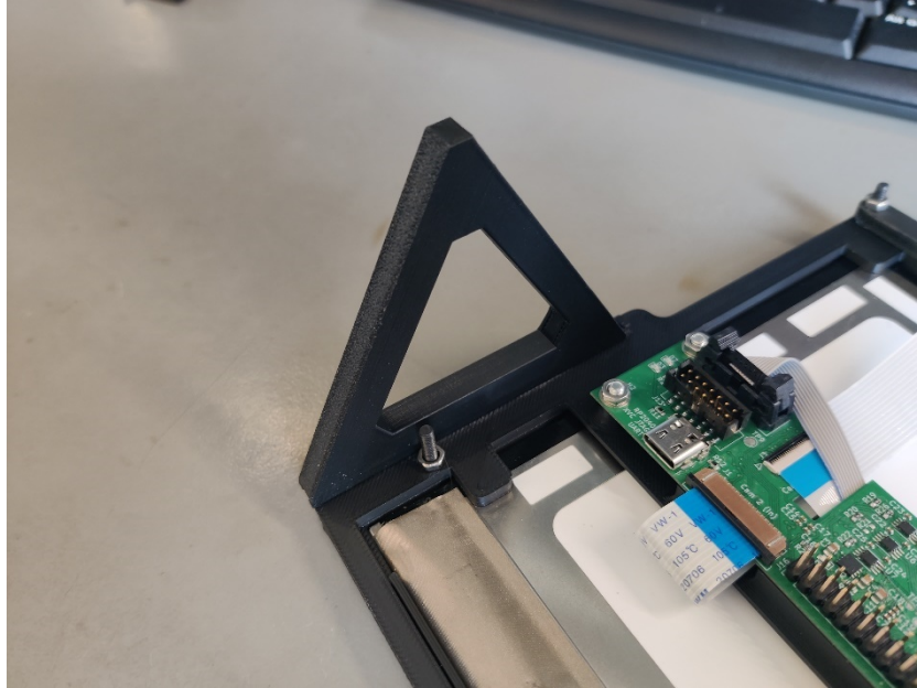
Figure 30: One of the legs attached to the Frame
